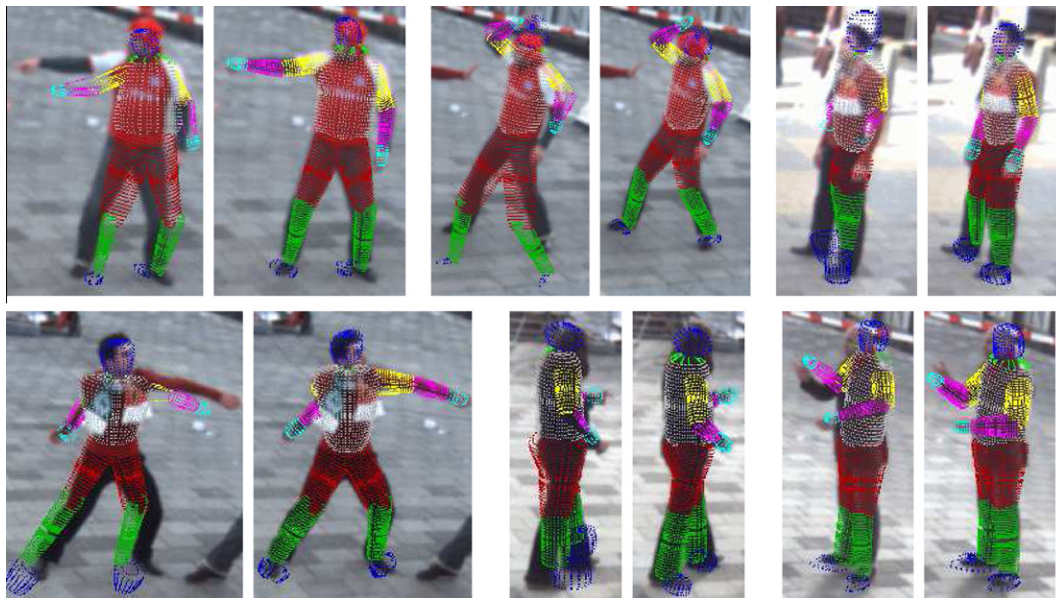
Fig. 7. Before and after model/pose adaptation. Reduction of avg. pose vertex error from 8.7 → 3.8, 16.1 → 5.0, 8.6 → 3.8, 8.8 → 3.8, 8.1 → 4.2, 10.1 → 4.9 (in cm, from left to right, 1 st and 2 nd row).
