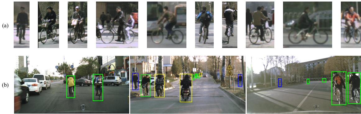
Fig. 4. Overview of the new cyclist detection dataset. (a) Cyclist samples; (b) Test images with annotations: green, blue and yellow bounding boxes indicate cyclists, pedestrians and other riders respectively.
