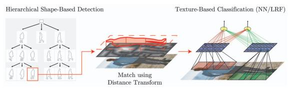
Fig. 5. Overview of combined shape-based detection and texture-based classification.
