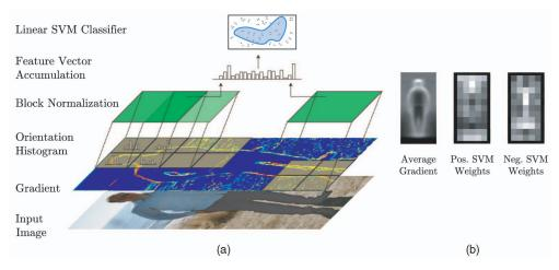
Fig. 4. (a) Overview of HOG/linSVM architecture. Cells on a spatial grid are shown in yellow, whereas overlapping normalization blocks are shown in green. (b) Average gradient image along with visualization of positive and negative SVM weights, which highlight the most discriminative regions for both the pedestrian and nonpedestrian classes.
