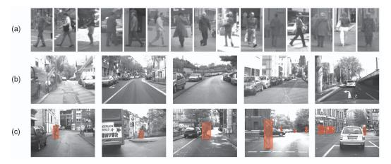
Fig. 1. Overview of the Daimler pedestrian detection benchmark data set: (a) Pedestrian training samples, (b) nonpedestrian training images, (c) test images with annotations.
