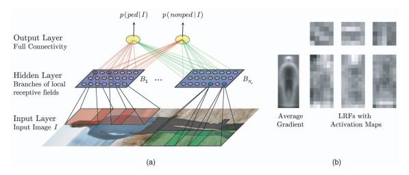
Fig. 3. (a) Overview of NN/LRF architecture. (b) Average gradient image along with three exemplary  $5 \times 5$ -pixel local receptive field features (hidden layer weights) and their activation maps (output layer weights) for the "pedestrian" output neuron, highlighting regions, where corresponding LRFs are most discriminative for the pedestrian class.
