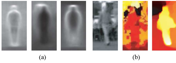
Fig. 2. (a) Average gradient magnitude of all pedestrian training samples for intensity, depth, and motion (left to right). (b) A difficult-to-recognize (low-contrast) pedestrian in the intensity domain can be very salient in other modalities.
