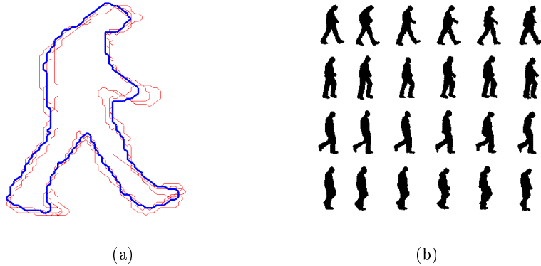
Fig. 6. (a) Computing a "mean" or prototype shape (in black) from aligned shape samples (in grey) (b) Shape clustering: each row contains the elements of a different cluster
