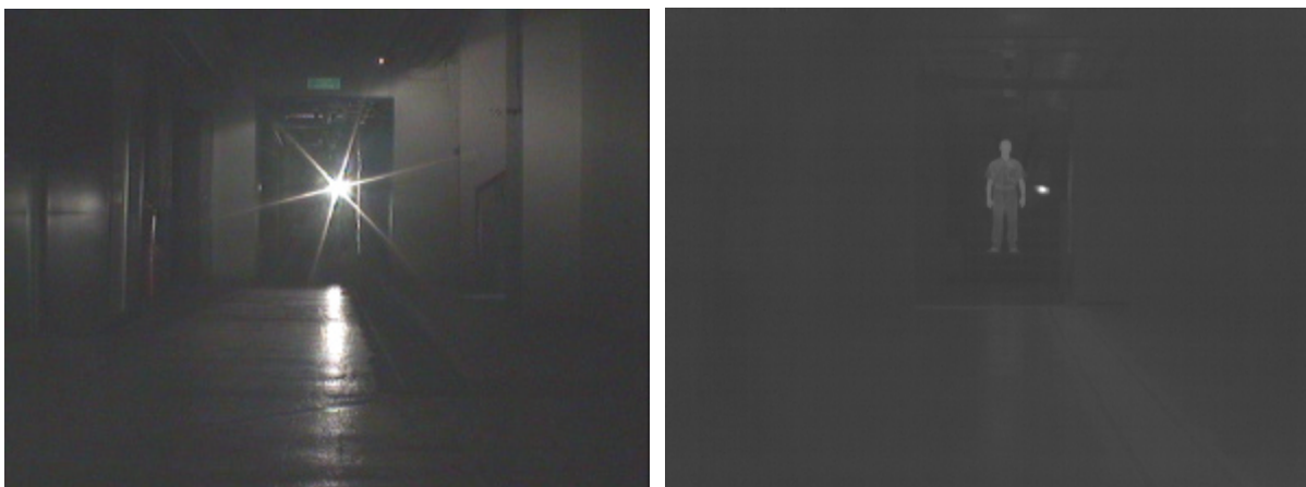
Figure 1: Car back-lighting (simulation of a pedestrian wearing light colour clothes by a clear night enlightened by car dipped headlights and with a front headlight)
