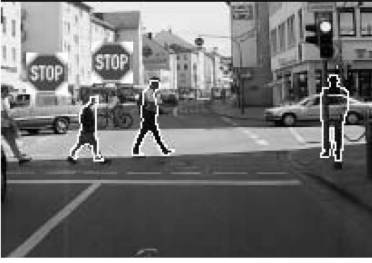
Fig. 16. Pedestrian classification—detections shown in white, solutions classified as pedestrians marked by STOP sign.
