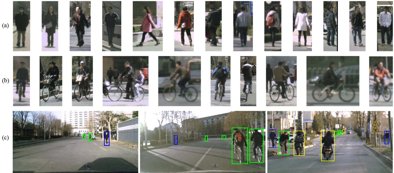
Fig. 8. Overview of the new pedestrian and cyclist detection dataset. (a) Pedestrian samples. (b) Cyclist samples. (c) Test images with annotations: Blue, green, and yellow bounding boxes indicate pedestrians, cyclists, and other riders, respectively.
